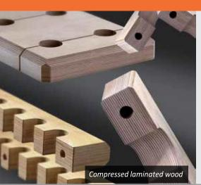
Compressed laminated wood is made of layers of wood veneer that are coated or impregnated with a synthetic resin and then pressed together under high pressure and temperature. Owing to its special material properties, compressed laminated wood is used primarily in the transformer industry and as a means of thermal insulation in machines and electrical systems.
